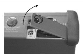
Figure 6. Removing the Battery Access Door
