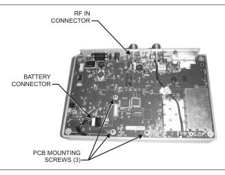
Figure 15. Main PCB (shown with optional T1/E1 PCB installed)
