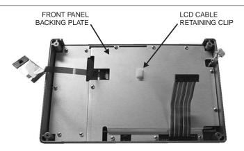
Figure 12. Front Panel Backing Plate
