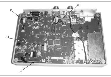
Figure 11. Site Master Front Panel Cable Connections
