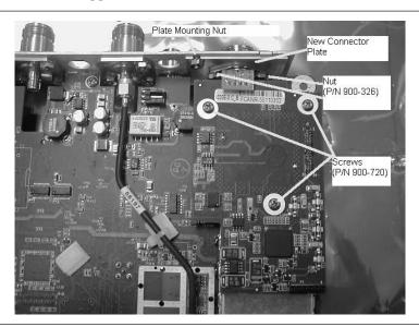
Figure 17. Power Monitor PCB Assembly Replacement
