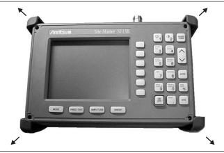
Figure 9. Removing the Corner Bumpers
