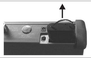
Figure 7. Removing the Battery
