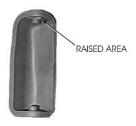
Figure 10. Corner Bumper Detail
