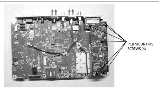
Figure 18. T1/E1 Tester PCB
