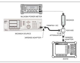
Figure 3. Power Meter Verification Setup
