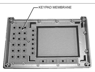
Figure 14. Front Panel Keypad Membrane
