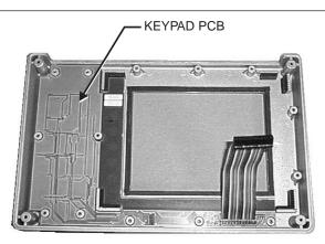
Figure 13. Front Panel Keypad PCB Location
