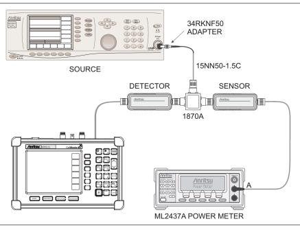
Figure 1. Power Monitor Verification Setup
